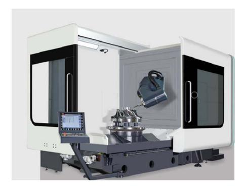
Use the telescopic cover and protective sheet metal to protect the chips generated during operation, avoid cutting splashes and cause damage to other mechanisms
